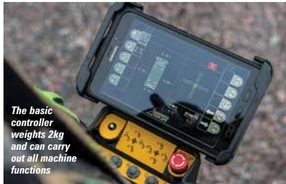
A tablet type screen can be integrated with the controller
