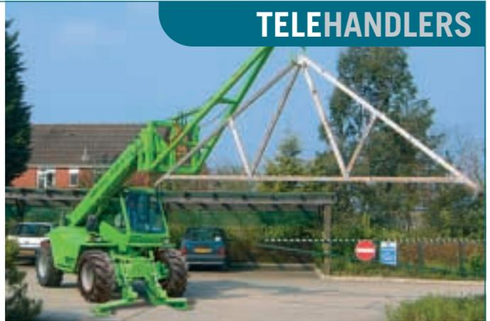
Merlo has introduced attachments specifically designed to permit its telehandlers to travel with the boom lowered while transporting roof trusses on site.
