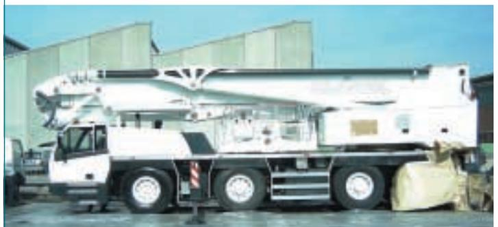
The latest truck mount from Oil & Steel, launched at Intermat, is its 76 metre working height Stargate 7638. The unit is mounted on a 4-axle, all-steer chassis and provides a 38 metre working radius.
