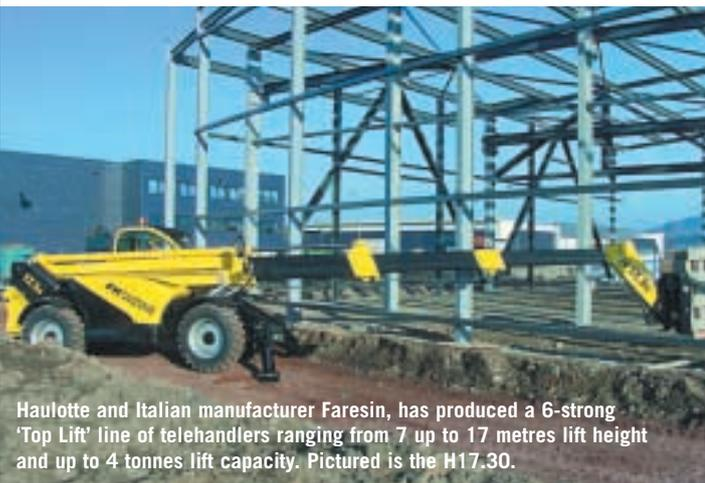
**Haulotte and Italian manufacturer Faresin, has produced a 6-strong 'Top Lift' line of telehandlers ranging from 7 up to 17 metres lift height and up to 4 tonnes lift capacity. Pictured is the H17.30.**
