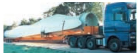
A COLLABORATIVE effort between Broshuis and specialists in windmill transportation, Carden of Denmark, and Germany’s Schaumann Schwertransport has resulted in The Triple Wing Trailer. The model is a hybrid of Broshuis’ platform Triple Trailer and its semi Triple Trailer, combining the manoeuvrability of the Triple Trailer’s steering characteristics and the low loading platform height of the semi Triple Trailer.
