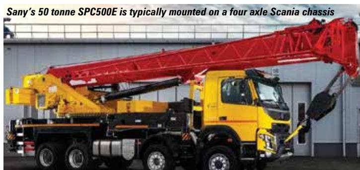
**Sany's 50 tonne SPC500E is typically mounted on a four axle Scania chassis**
