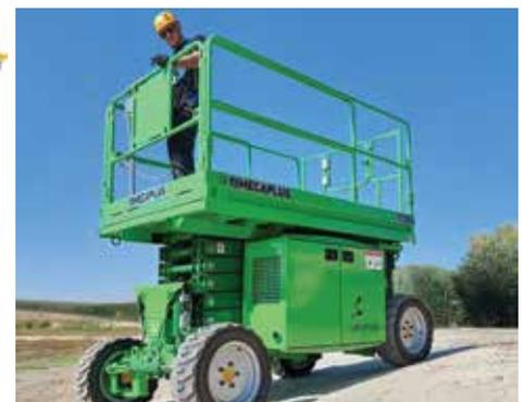
Spanish manufacturer **Mecaplus** delivers its first 34ft T12SL 4x4 self-levelling scissor lift.
