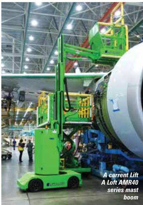
A current Lift A Loft AMR40 series mast boom
