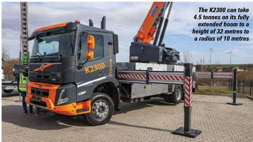
*The K2300 can take 4.5 tonnes on its fully extended boom to a height of 32 metres to a radius of 10 metres*
