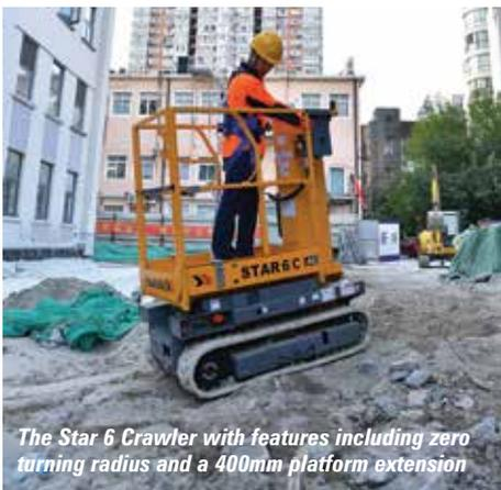
The Star 6 Crawler with features including zero turning radius and a 400mm platform extension
