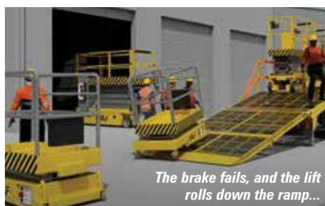
The brake fails, and the lift rolls down the ramp...
