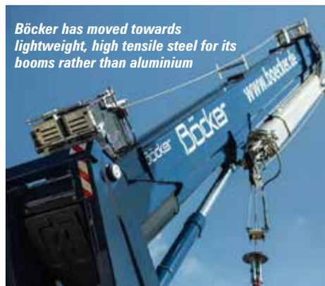
*Böcker has moved towards lightweight, high tensile steel for its booms rather than aluminium*
