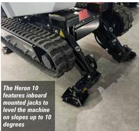
The Heron 10 features inboard mounted jacks to level the machine on slopes up to 10 degrees
