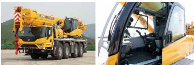
the maximum counterweight is 20 tonnes. The crane can travel with either nine tonnes of counterweight and hook blocks within 12 tonne axle loads, or seven tonnes plus the bi-fold extension and block. Axle loads with all 20 tonnes of counterweight on board are 15.5 tonnes.
