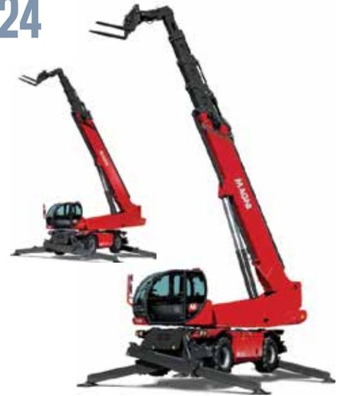
**Magni** unveils two heavy duty, eight tonne capacity 360 degree telehandlers - the 35 metre RTH8.35 and the 46 metre RTH8.46.
