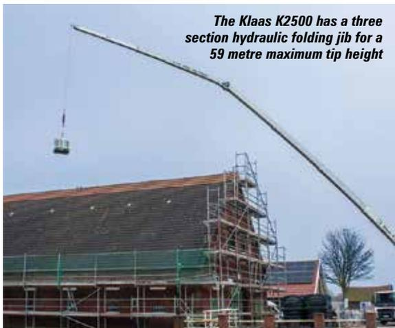
*The Klaas K2500 has a three section hydraulic folding jib for a 59 metre maximum tip height*
