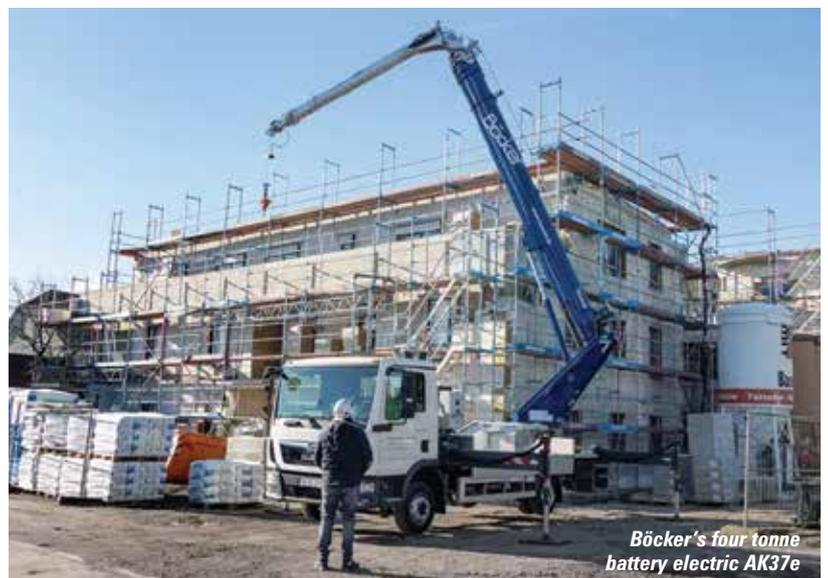
Böcker's four tonne battery electric AK37e
