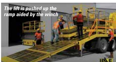
The lift is pushed up the ramp aided by the winch
