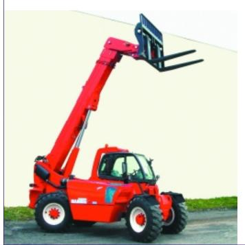
MANITOU HAS expanded its range of heavy-duty telescopic trucks with the introduction of the MHT 10120 L Turbo. The 10 tonne capacity unit sits midway in Manitou's existing four-strong heavy-duty line with capacities ranging from 6.5 to 16 tonnes. The 9.8 metre working height MHT 10120 L is fitted with a 170 horsepower Mercedes Turbo engine and features hydrostatic transmission, four drive and steerable wheels and crab steering.
