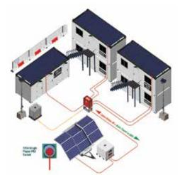
should be capacity (kWh) and the output (kW) needed on the site from the electrical requirement, the type of electrical load, and its geographical set up.
