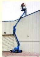
AB38 electric Lite, the new bi-energy features a 1.5 metre wide chassis, a 0.4 metre turning circle and 36 per cent grade-
