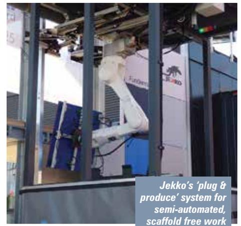
*Jekko's 'plug & produce' system for semi-automated, scaffold free work on building façade refurbishment being operated at Bauma*
