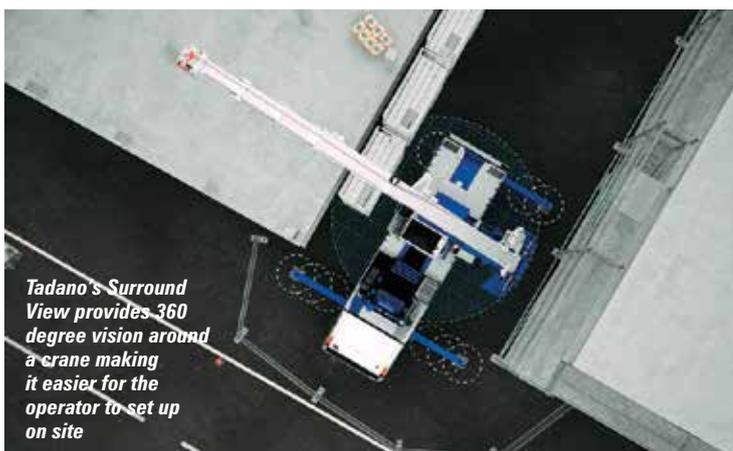
*Tadano's Surround View provides 360 degree vision around a crane making it easier for the operator to set up on site*
