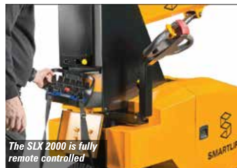
The new Smartlift SLX 2000 has a lift capacity of 1,000kg, lift height of 5.25 metres and 2.75 metres of forward reach
