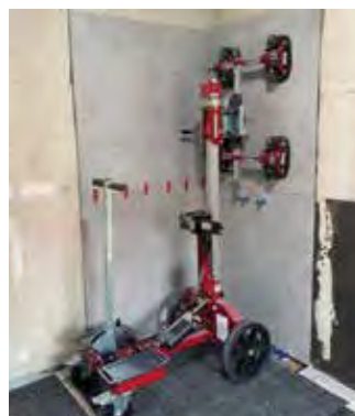
The battery powered Winlet 785 with wired remote control combines a pick & carry crane ability for glass panels up to 785kg
