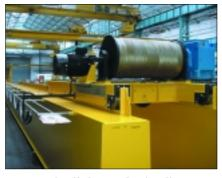
Fresh off the production line. Morris Material Handling is supplying two, 20 tonne Goliaths to an undisclosed customer. The two units are designed to run in tandem allowing the customer to handle containers up to 12.2 metres
