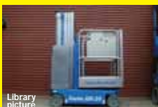
GENIE RUNABOUT GR20 (2006) Self propelled personnel lift. 26' working height. Battery. Serviced & tested.
