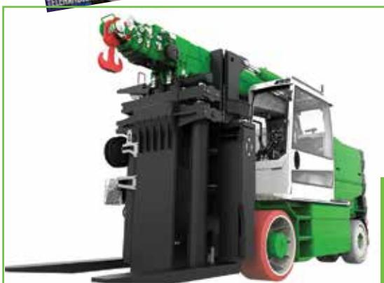
**JMG** unveils its first hydrogen hybrid pick & carry heavy forklift/crane using a 96V hydrogen fuel cell module fed by a 6kg hydrogen gas tank.
