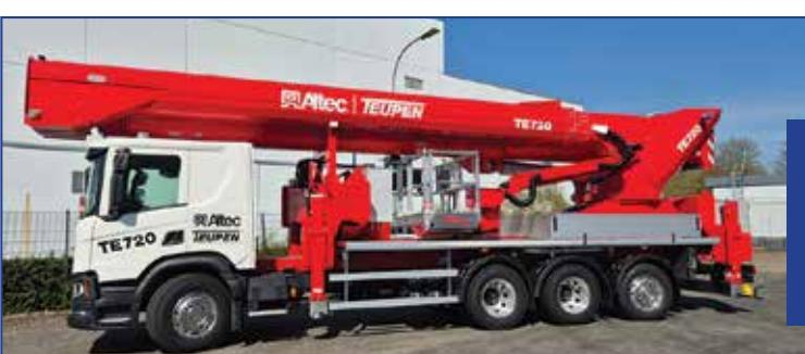
Two new 70 metre plus truck mounted lifts - **Altec Teupen's** 72 metre TE720 and **Multitel's** 70.6 metre MJE710 - are unveiled at Bauma.
