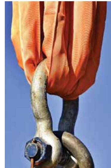
Wide body shackles significantly reduce this effect by increasing the bearing radius and improving load distribution. For many lifts, using a wide body shackle is the single most effective way to reduce sling damage.
