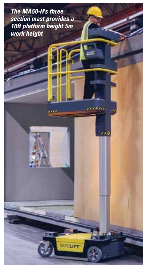
The new Safelift MA50-H in self-propelled mode
