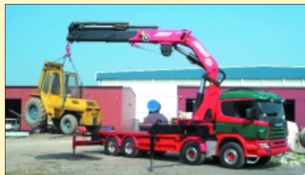
R.S. French of Faversham in Kent has recently taken delivery of this PM 75026 SP with 16 metres of horizontal outreach at which it can lift 3500Kg. Features of the crane include Continuous slew via two reduction gearbox/motor, radio remote control, Danfoss valve block, Twin linkage and 8780mm stabiliser spread. Approximate cost of the crane is £150,000 – PM has already sold eight of them this year.
