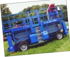
water positioned on one side to simulate the weight of a man. The platform was then raised to its maximum height (using ground-level controls) to allow measurement of divergence from the vertical.
