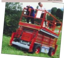
the "innards" was good and, as on most of the larger machines, the motor slid out for easy maintenance. Scissor protection is provided by a lattice grille.
