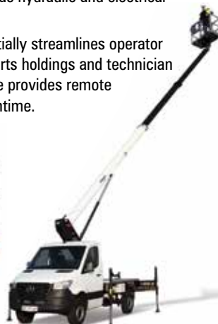
The new 20 metre V-200 is one of the new V-Range of 3.5 tonne mounted lifts from Time Versalift
