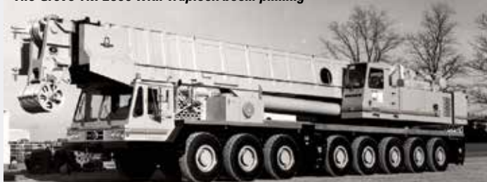
The Grove TM 2500 with Traplock boom pinning
