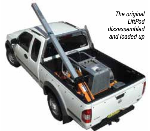
The smaller 3.8 metre working height FS60 LiftPod
