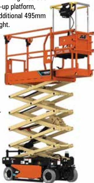
JLG's new 26ft micro scissor lift, the ES2632M with step-up platform
