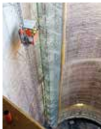
The Vectio 350 personnel and material transport platform is available in six sizes ranging from 500kg to 2,000kg capacity
