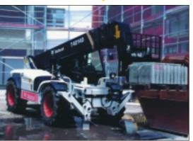
Telescopic handlers with lift capacities from 2.5 to 4 tonnes and lift heights from 5.6 to 17 metres.
