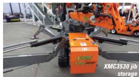
The new crane fully stowed - note the two counterweights
