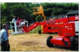
that of ours. The exceptionally high figure of 114 seconds for elevating speed is partially explained by the fact that this is a larger machine than the others and has about a metre more of boom. A final difference is that Snorkel describes the standard machine's slewing as being "continuous" – the particular model that we tested was being delivered the next day to a customer that had specified 358 degrees slewing.
