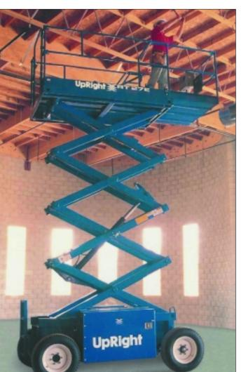
The new XRT27E (10.2m/33 ft working height) and XRT33E (11.8m/39 ft working height) are electric scissors with very powerful offslab capabilities for work on ground conditions which would defy the conventional electric slab scissor and many 4x2 diesel scissors
