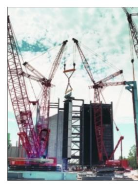
The Model 21000 is Manitowoc's largest crane. Its maximum reach is 195 meters (640 feet) when fitted with 340 feet of boom and 300 feet of luffing job. The Max-er attachment boosts the crane's capacity to 907 metric tons (1,000 tons). A feature of the crane is its variable stance which is made possible by the patented Octatrac eight-crawler system that can be configured to narrow its stance from 46 feet to 30 feet.
