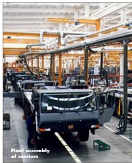
other vital components. The design of the plant allows these to be delivered to the precise section of the assembly line that needs them: "the principle is for production material to reach the assem-
