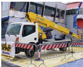
Leader claims to have taken 100 orders for its 20 metre Jet 200 truck mounted lift. The unit has many innovative features including the jib which can be retracted into the main boom for travel and to create a regular straight boom while the turret pivots, with a hydraulic cylinder to improve outreach and incorporates the lift's overload sensor.
