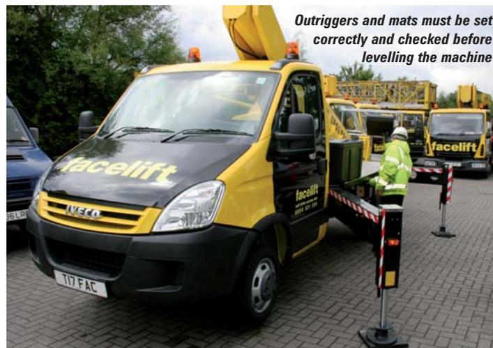
*Outriggers and mats must be set correctly and checked before levelling the machine*
