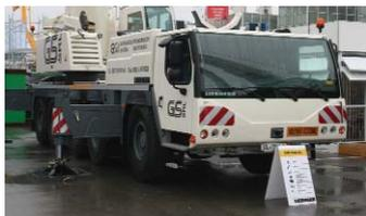
For many, this was their first sight of the 130 tonne capacity Liebherr LTM 1130 5.1. The unit has a 60 metre main boom with the addition of up to a 19 metre swing away extension and two seven metre long lattice sections. The unit has a 12.26 metre long chassis and is 2.75 metres wide. Other features include active speed-dependent rear axle steering, air operated disc brakes and a 370kW (503hp) Tier 3 engine.
