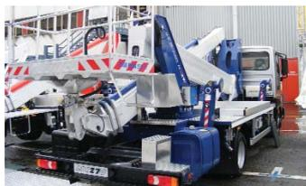
A new articulated truck mounted boom from Multitel Pagliero - the MX270D - extends the MX range to 27 metres. The unit seen at the show was mounted on a 5.6 tonne chassis to meet Italian self-drive rules and offered 13 metres outreach. The platform will be mounted on a Mitsubishi Canter 7.5 tonne chassis in the UK and should be available at the beginning of 2008 at an attractive price.
