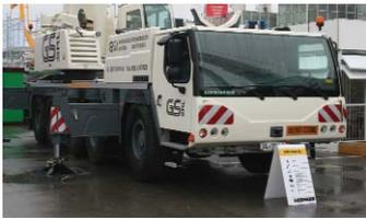
For many, this was their first sight of the 130 tonne capacity Liebherr LTM 1130 5.1. The unit has a 60 metre main boom with the addition of up to a 19 metre swing away extension and two seven metre long lattice sections. The unit has a 12.26 metre long chassis and is 2.75 metres wide. Other features include active speed-dependent rear axle steering, air operated disc brakes and a 370kW (503hp) Tier 3 engine.
