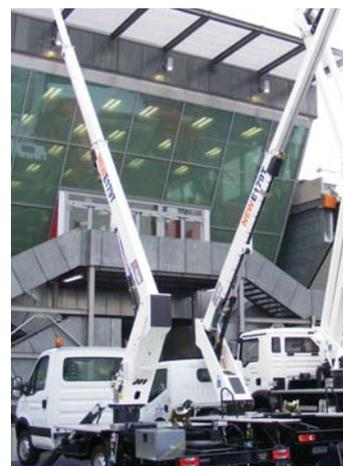
GSR introduced a new 17 metre telescopic boom - the E179T. Mounted on a 3.5 tonne truck the unit is capable of 12 metres outreach.
