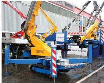
Not currently available in the UK - mainly the Middle East and North Africa - are the co.me.t truck mounted and spider machines. The company produces three crawler models - 12 metre, 16 metre and 18 metre. It was also showing a new 19 metre, 3.5 tonne truck mounted Eurosky AT.
