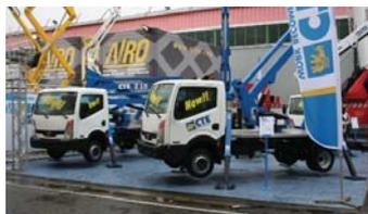
CTE launched several new truck mounted platforms including the 20.8 metre working height Z21 and the 19 metre, 230kg capacity Z19.
