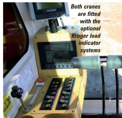
Both cranes are fitted with the optional Kruger load indicator systems
