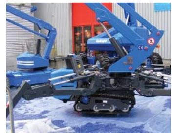
Leader also showed a 16 metre spider lift called the Jumper 160, the first two of which have been sold in Holland. The new model features an unusual crawler chassis with a raised drive sprocket and pinion mounted bottom rollers which allow the lift to travel over obstacles without the mid track tip problem that occurs on many tracked machines.
