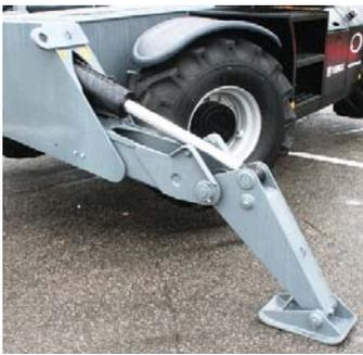
Terex was showing its new stabiliser system for its telehandlers.
