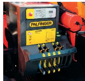
*The easier to use Palfinger control panel.*
