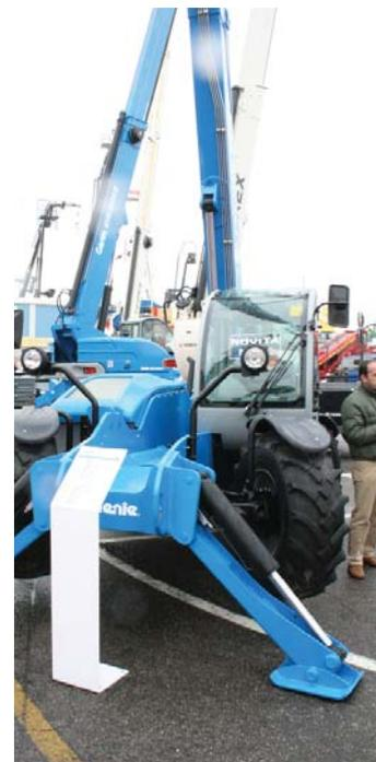
Genie has introduced the the GTH4017SX - a lower cost, simpler machine aimed specifically at the rental market.
