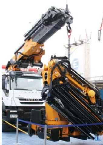
Effer unveiled two new loader cranes: The, 92 tonne/metre Effer 1355/9S (mounted) features X-type outriggers which keep the sub-chassis shorter and also gives a better load slewing range. Being lifted is the 470/6S - a six extension unit with a 41.6 tonne/metre capacity and an outreach better than 26 metres.
