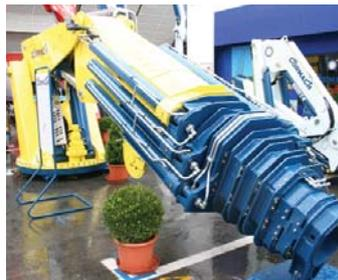
A massive new 200 tonne/metre articulated loader crane from Cormach - the 225000 E9 - has been designed specifically for industrial moving. The nine section beast has a 45 tonne lift capacity at 4.5 metres and is capable of lifting 6.1 tonnes at 23 metres and taking more than a tonne out to 42 metres.
