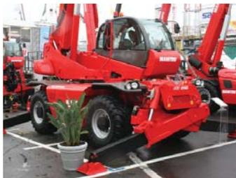
Several new Privilege series from Manitou were on the stand including the roto MRT 2150 (above) which can lift up to five tonnes to 20.6 metres, and the MRT 3050 which can take the same load to 29.7 metres. Largest machine on the stand was the 21 tonne capacity MHT 10210.
