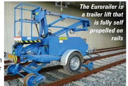
The Eurorailer is a trailer lift that is fully self propelled on rails
