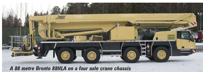
*A 88 metre Bronto 88HLA on a four axle crane chassis*
